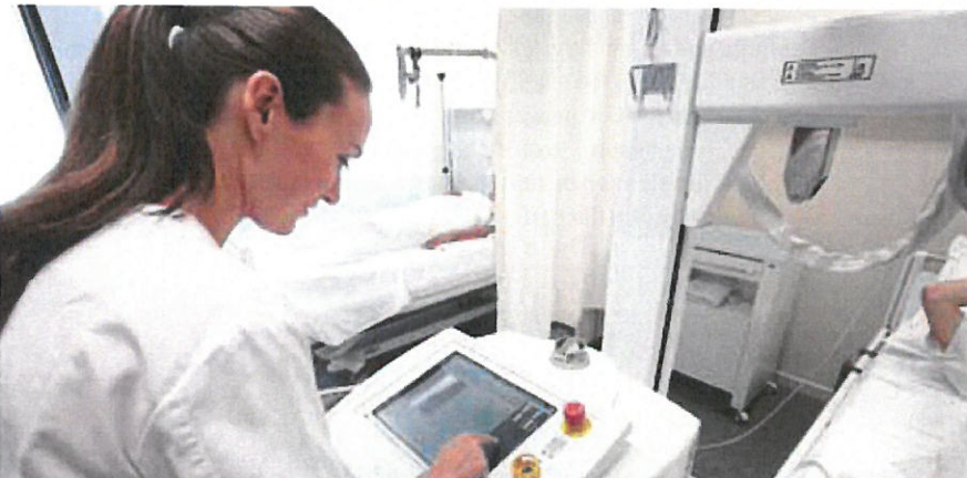
Immediate image capture at patient's bedside. System incorporates fully integrated NX acquisition workstation touch screen
